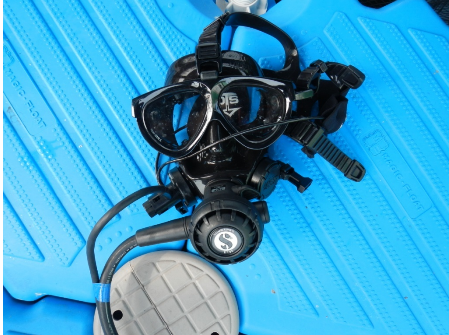
Figure 7. The full face mask utilized is the 'Manta' from OTS. It will accept any standard 2nd stage regulator.
