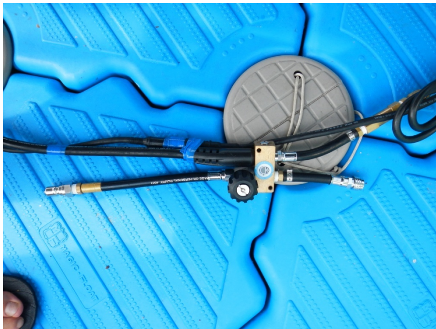
Figure 8. The diver-worn bailout cylinder connects to the bailout whip at the manifold block. This is a standard Parker QC fitting used in commercial diving. The isolation valve should be 'off' while diving. If the surface supplied air supply fails, the diver can open this valve and have immediate access to the reserve air on his/her back. The dive should be terminated immediately.
