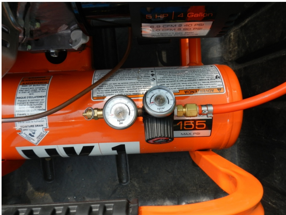
Figure 12. The outlet pressure on the compressor should be adjusted to supply 120-150 psi to the divers.
