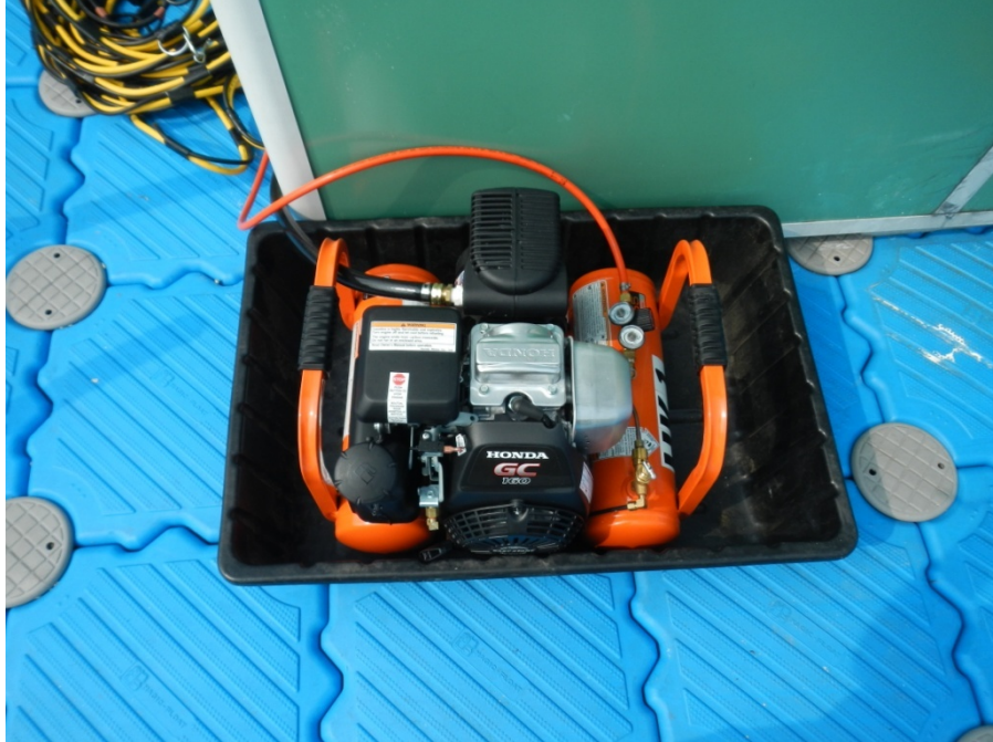
Figure 11. The compressor rests in a spill pan to mitigate accidental gas spills. This should always be run in a well ventilated area.
