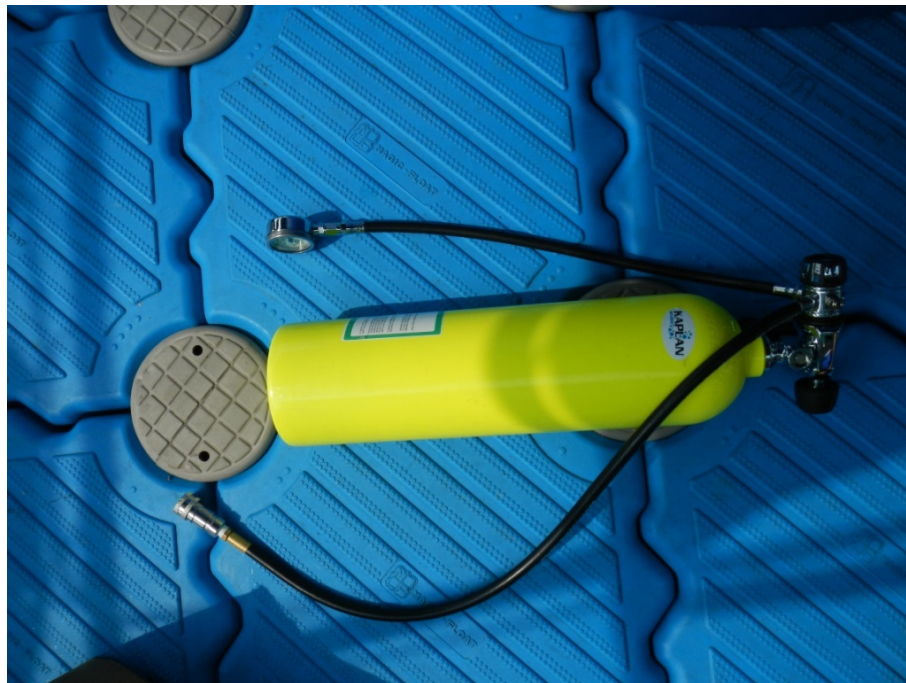
Figure 10. The diver-worn bailout cylinder is worn inverted with the bailout whip coming over the divers left shoulder. The cylinder should be 'on' during the dive, but is only utilized in an emergency. The diver should be able to reach back and actuate this valve unassisted.
