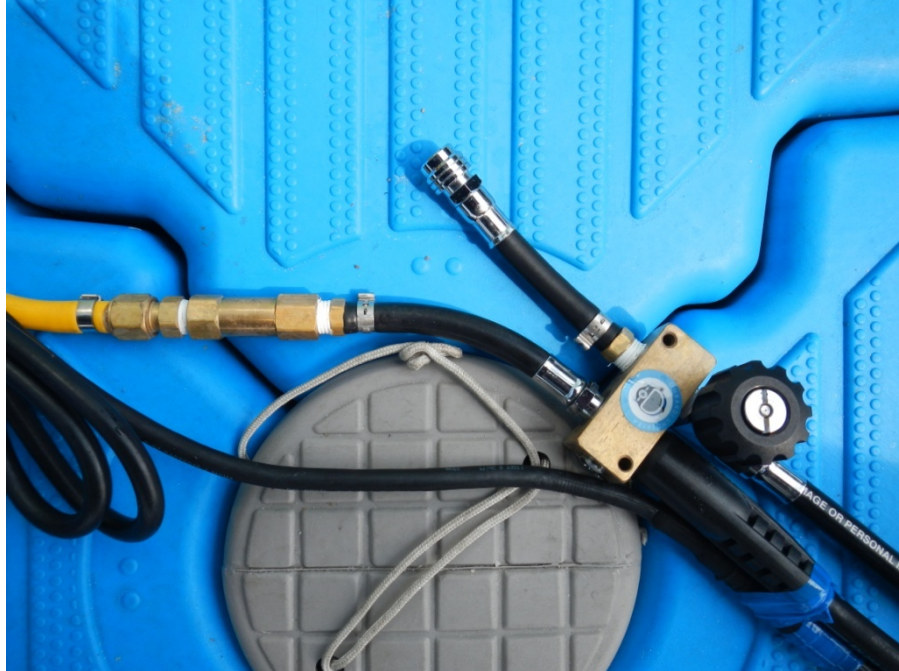
Figure 9. The air supply/umbilical attaches to the manifold at a check valve. This prevents the backflow of gas if the umbilical is severed. A short inflator hose fits to the BC inflator at the diver's left chest and positions the manifold block at the left shoulder for immediate access. The LP breathing hose routes around the diver's neck with air supplied over the right shoulder as is standard for scuba equipment.
