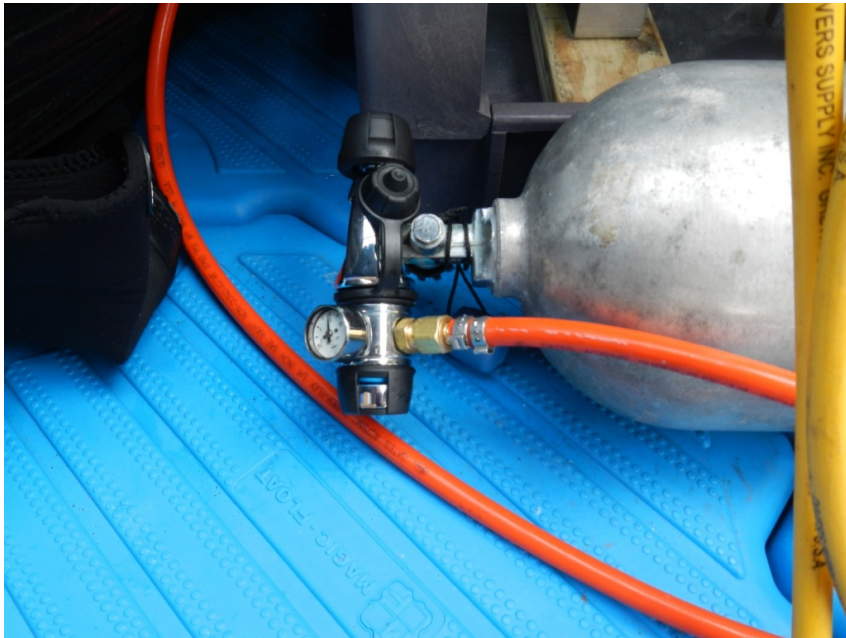
Figure 3. The HP bailout is supplied through a first stage regulator. This includes an HP gauge and its own pressure relief valve. The supply hose is over-engineered to 2250psi however operates at only standard intermediate pressure. This is a failsafe to ensure air supply to the diver in an emergency. This cylinder should be 'on' during the dive, and isolated at the distribution manifold. Note that standard 'oxygen' brass fittings are used throughout the system. These are commonly used in commercial diving operations as they facilitate easy hose repair, and provide for readily available spares on-site.
